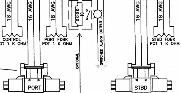
RELAY CONTACTS MUST BE ABLE TO HANDLE PUMPSET CURRENT. RELAY IS CUSTOMER SUPPLIED.
