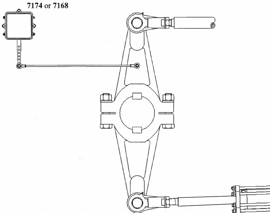
**IMPORTANT:** Hydraulic steering gears using a hydraulic Full Follow-Up System (often referred to as “Telemotor” or “Accumotor”) must drive the Feedback Unit from the Servo Cylinder, not the Rudder stock. In such a case, the Model 7174 Follow-Up should be mounted approximately two feet from the end of the Servo Cylinder. This is done to ensure proper linear motion. The cable for the Models 7174 or 7168 Feedback Unit should be a 3-conductor #18-gauge cable.
