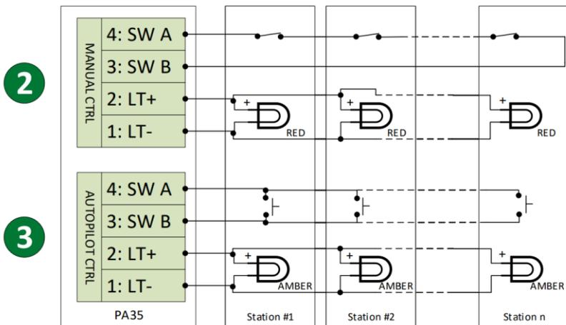
Figure 15: Multiple Station Control Panel Wiring
