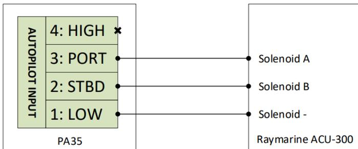
Figure 9: Example Autopilot Connection - Raymarine ACU-300
