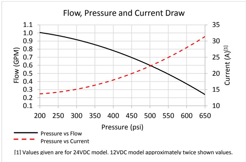
*Figure 2: PA35 Flow, Pressure, and Current Draw*
