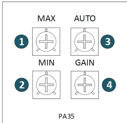
*Figure 18: Calibration Trimpot Arrangement
