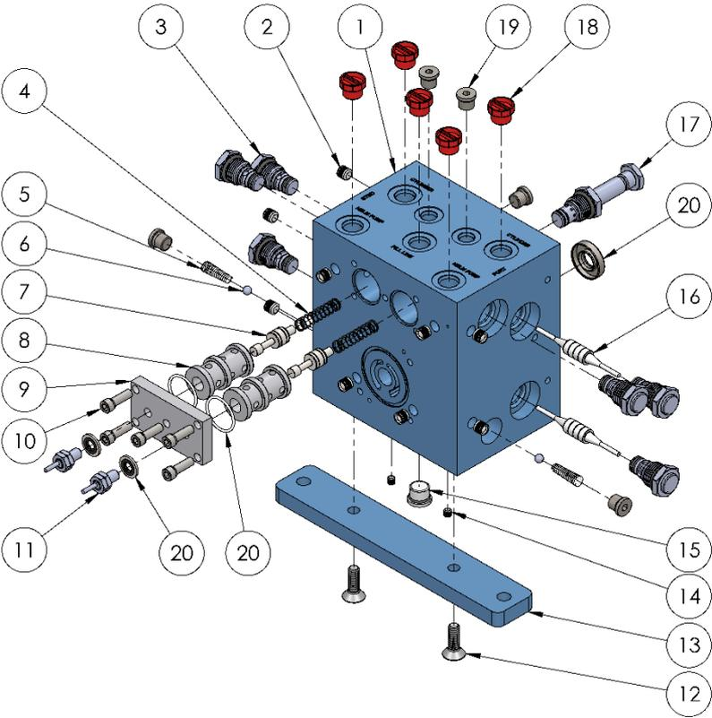
Figure 22: PA35 502-650 Manifold Parts Diagram
