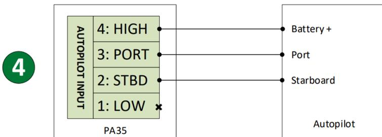
Figure 6: Generic Autopilot Wiring (Common Positive)
