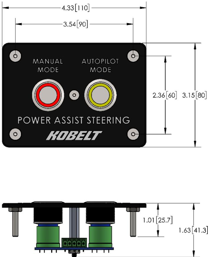
Figure 25: PA35 Control Panel Product Dimensions
