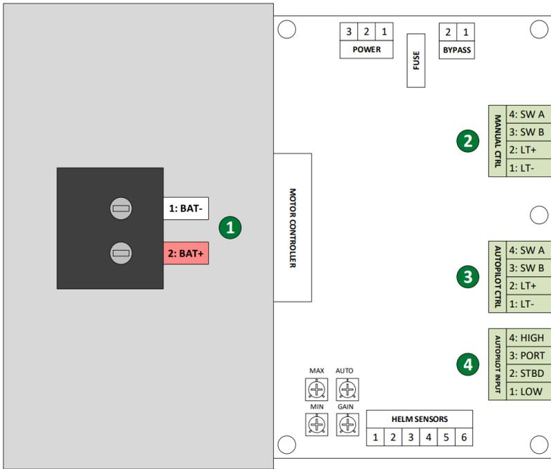
Figure 5: Internal PA35 Electrical Enclosure Connections
