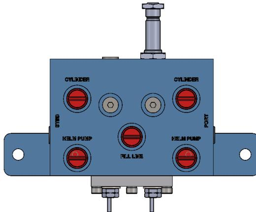
Figure 3: Connections in Top Face of Hydraulic Manifold
