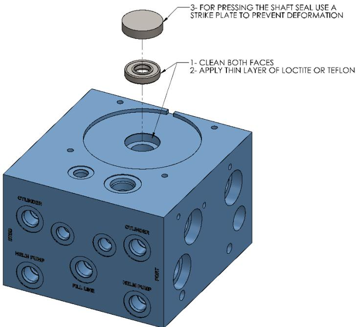
Figure 24: Motor Shaft Seal Diagram
