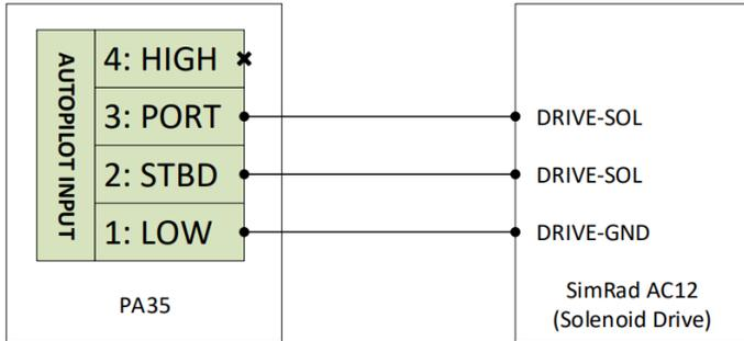
Figure 10: Example Autopilot Connection - SimRad AC12
