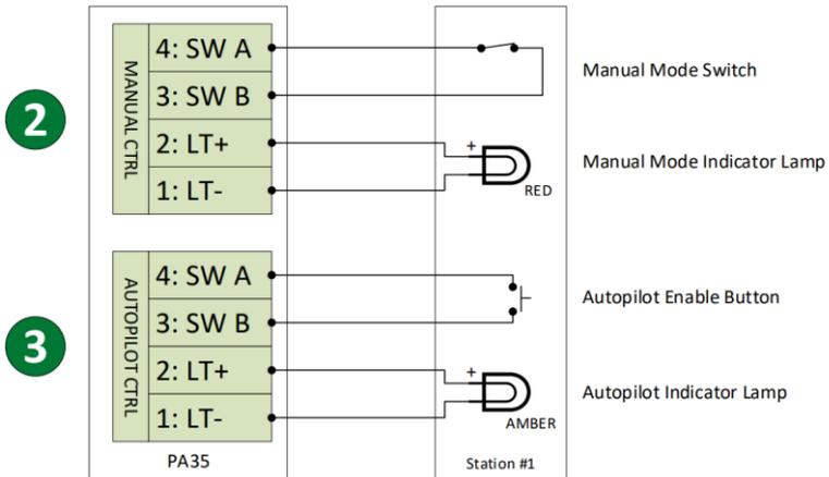
Figure 14: Single Station Control Panel Wiring
