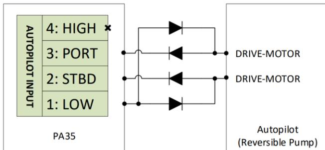
Figure 8: Generic Autopilot Wiring (Reversible Pump)
