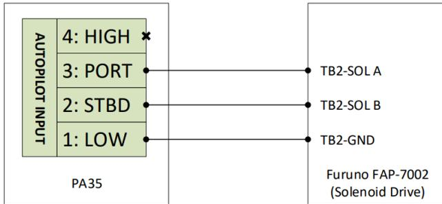
Figure 11: Example Autopilot Connection - Furuno FAP-7002
