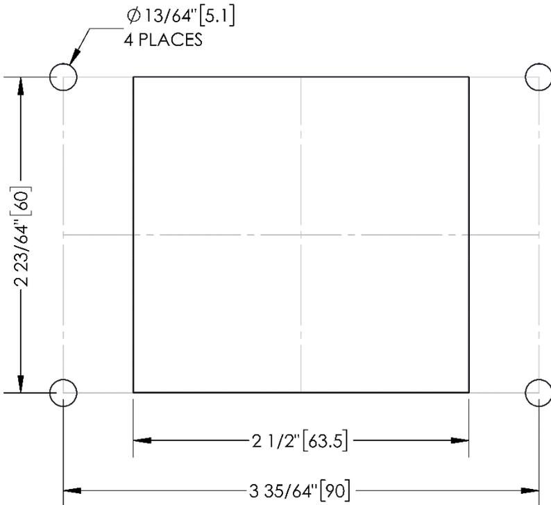
Figure 26: PA35 Control Panel Installation Cut-out Template
