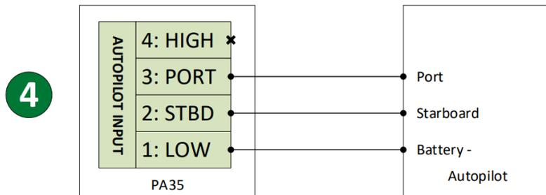
Figure 7: Generic Autopilot Wiring (Common Negative)
