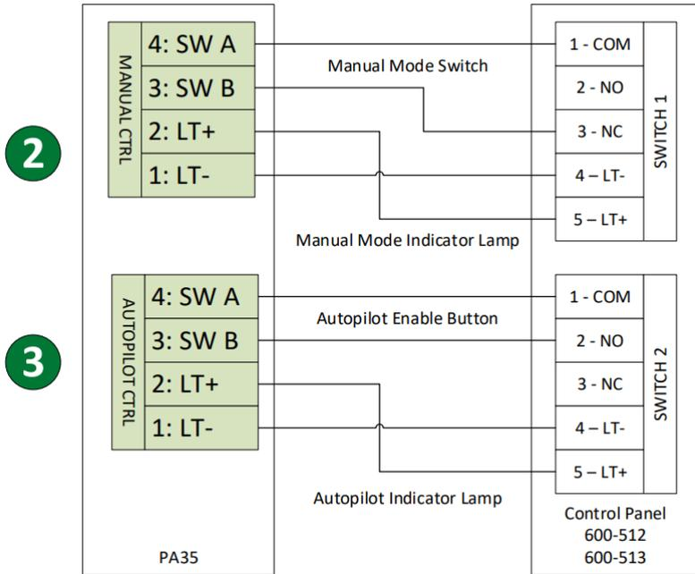
Figure 17: Kobelt PA35 Control Panel Wiring Diagram
