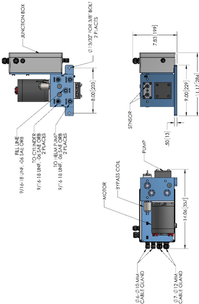
Figure 20: PA35 Installation Dimensions
