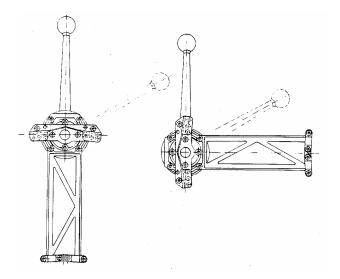
The above illustration shows two possible ways of connecting the cable lead to the side mount control.
