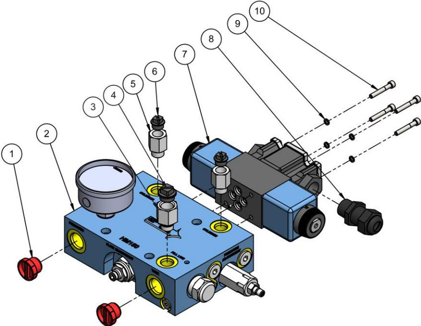
Figure 7: HM150 Parts Diagram
