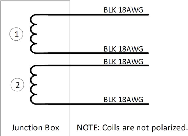
Figure 5: HM150 Electrical Wiring Diagram
