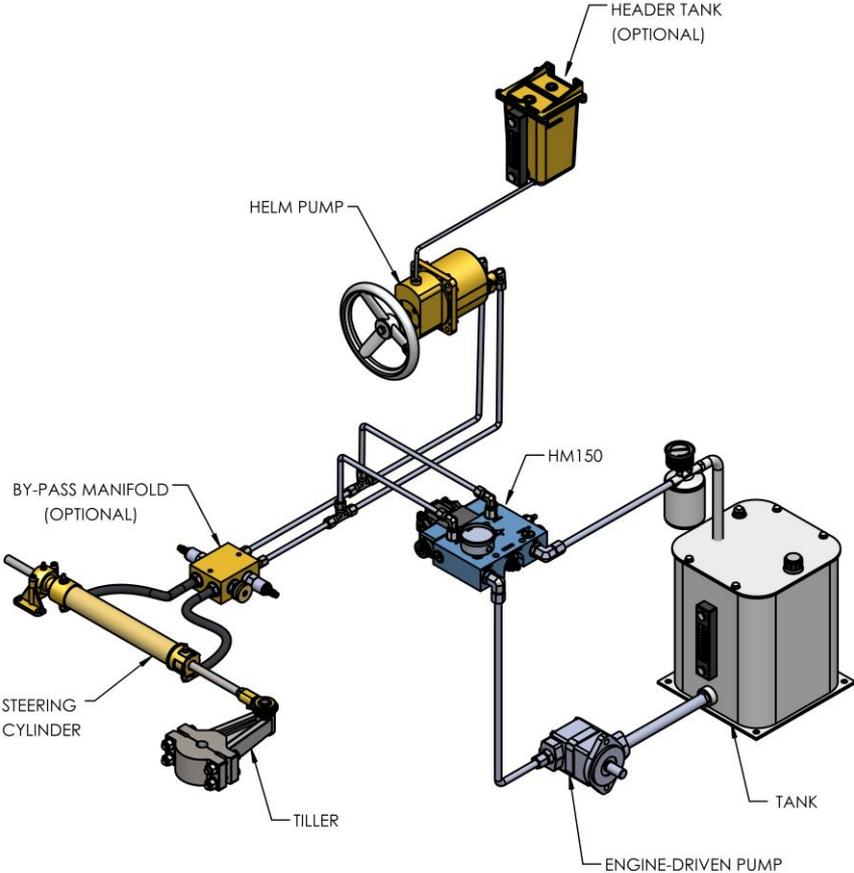
Figure 9: Typical System Arrangement
