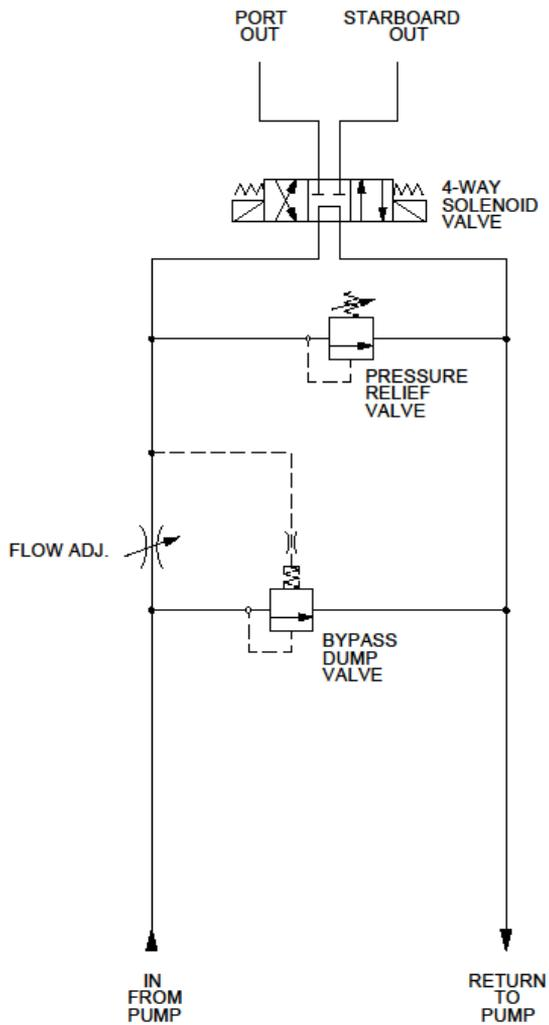
Figure 2: Hydraulic Schematic
