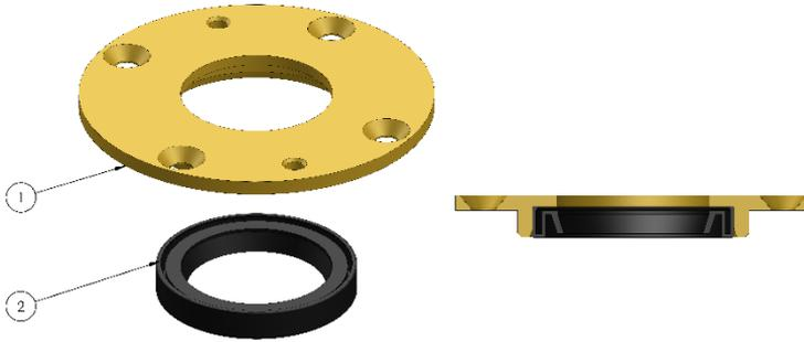
Figure 12: Front Seal Retainer sub-assembly
