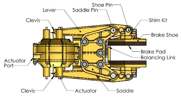
Figure 1: Caliper Brake Nomenclature
