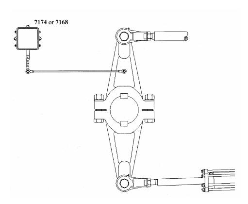
**IMPORTANT**: Hydraulic steering gears using a hydraulic Full Follow-Up System (often referred to as "Telemotor" or "Accumotor") must drive the Feedback Unit from the Servo Cylinder, not the Rudder stock. In such a case, the Model 7174 Follow-Up should be mounted approximately two feet from the end of the Servo Cylinder. This is done to ensure proper linear motion. The cable for the Models 7174 or 7168 Feedback Unit should be a 3-conductor #18-gauge cable.
