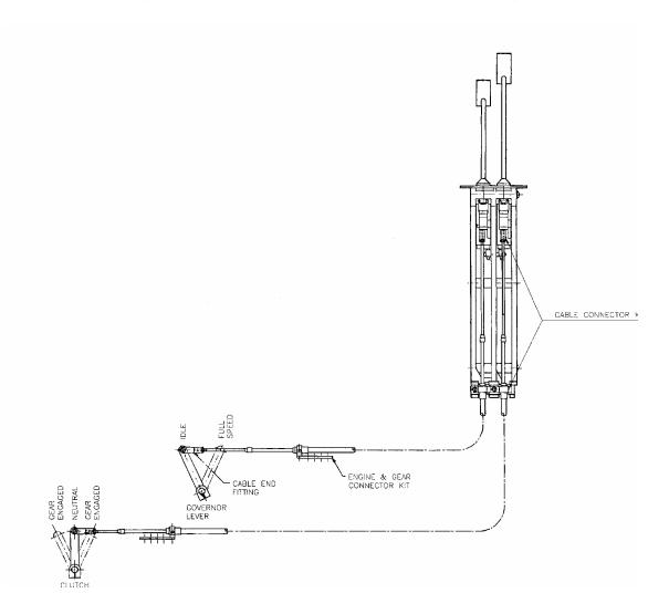
Recommended connection cables: Felsted cables 30 series or 40 series.
