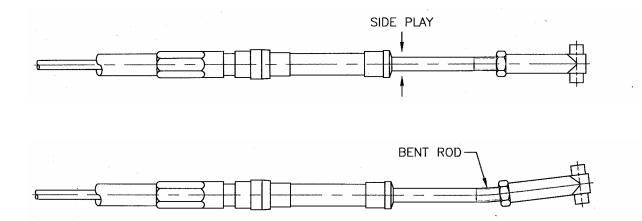
It is possible that a cable end may become bent either in transit during an installation or simply gets hit after it is installed. This, in fact, will also cause binding between the core rod and the sleeve.
