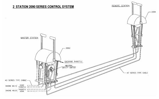
Push-Pull cables, Felsted 40 series cables, are used to connect the head to the engine clutch and throttle. 43 series are recommended. The installation instructions for the push-pull control cables are the same as the single lever control. Pull-Pull cables, needed to interconnect the control heads, should be installed last.
