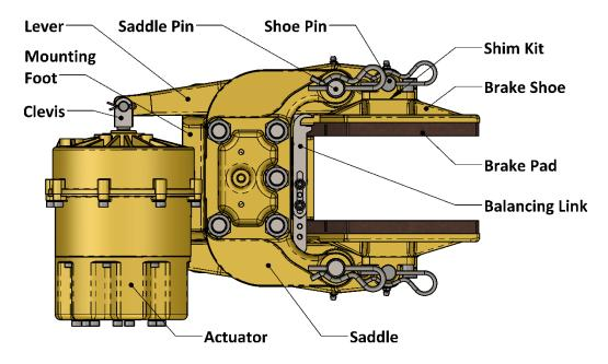
**Figure 1: Caliper Brake Nomenclature**
