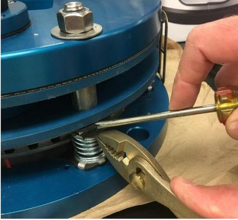
4. Remove all six pads on the mounting flange side.
