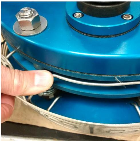
2. Starting with the mounting flange side pads first, push the pad retainer out of engagement with the backing plate. It may be necessary to use a brake spring plier or a screw driver.
