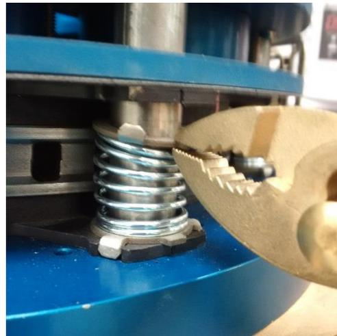
3. While holding the return spring compressed, slide the shoe radially outward. Repeat with the other retainer and lift the pad away.
