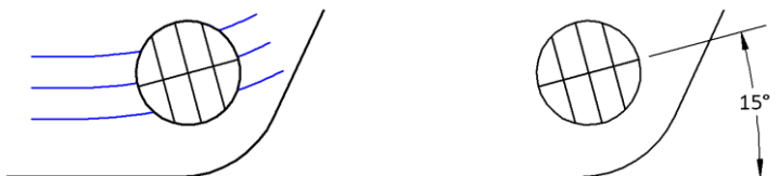
Figure 4 - Orientation of protective grid relative to vessel
