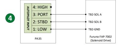
Figure 11: Example Autopilot Connection - Furuno FAP-7002
