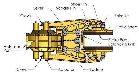
Figure 1: Caliper Brake Nomenclature
