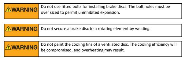
If the disc was damaged during installation with nicks or welding marks, remove the defects before putting into service.
