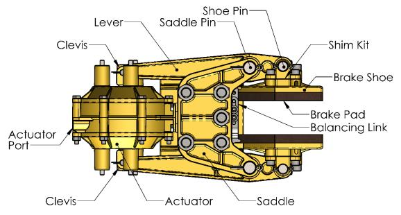
Figure 1: Caliper Brake Nomenclature
