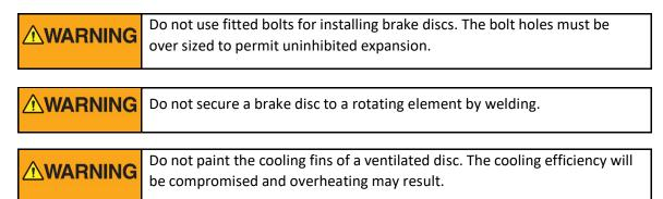
If the disc was damaged during installation with nicks or welding marks, remove the defects before putting into service.
