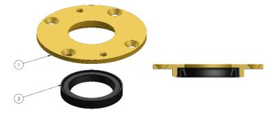
Figure 12: Front Seal Retainer sub-assembly
