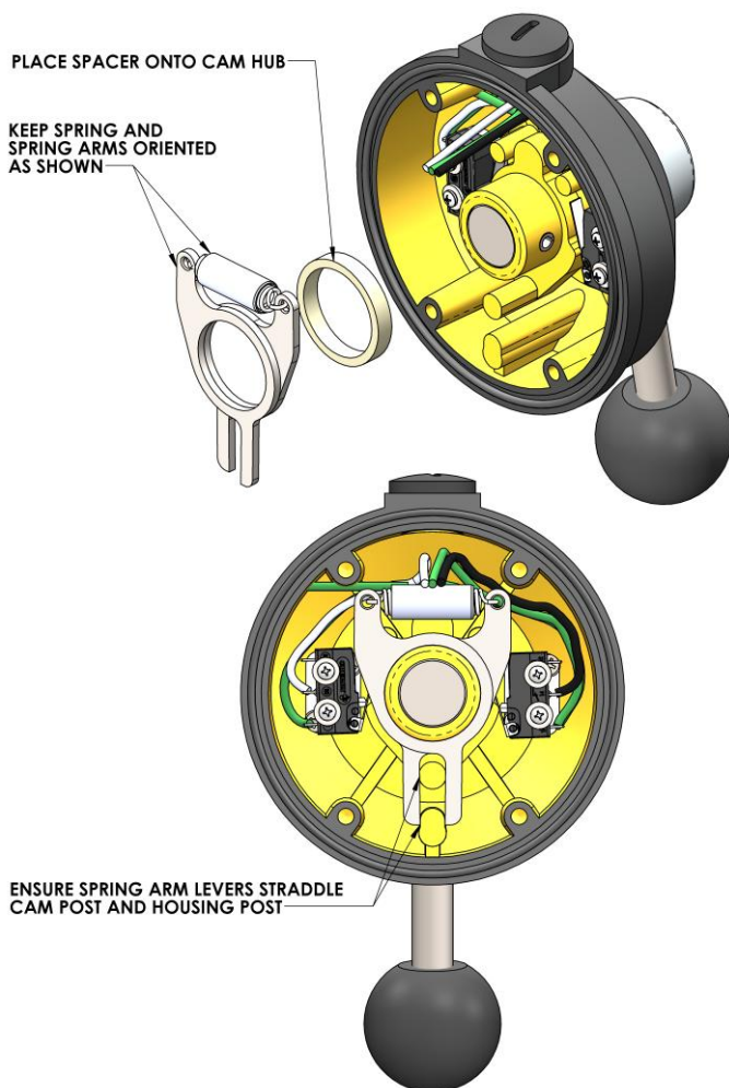
Figure 28: Installing spring assembly into jog housing.
