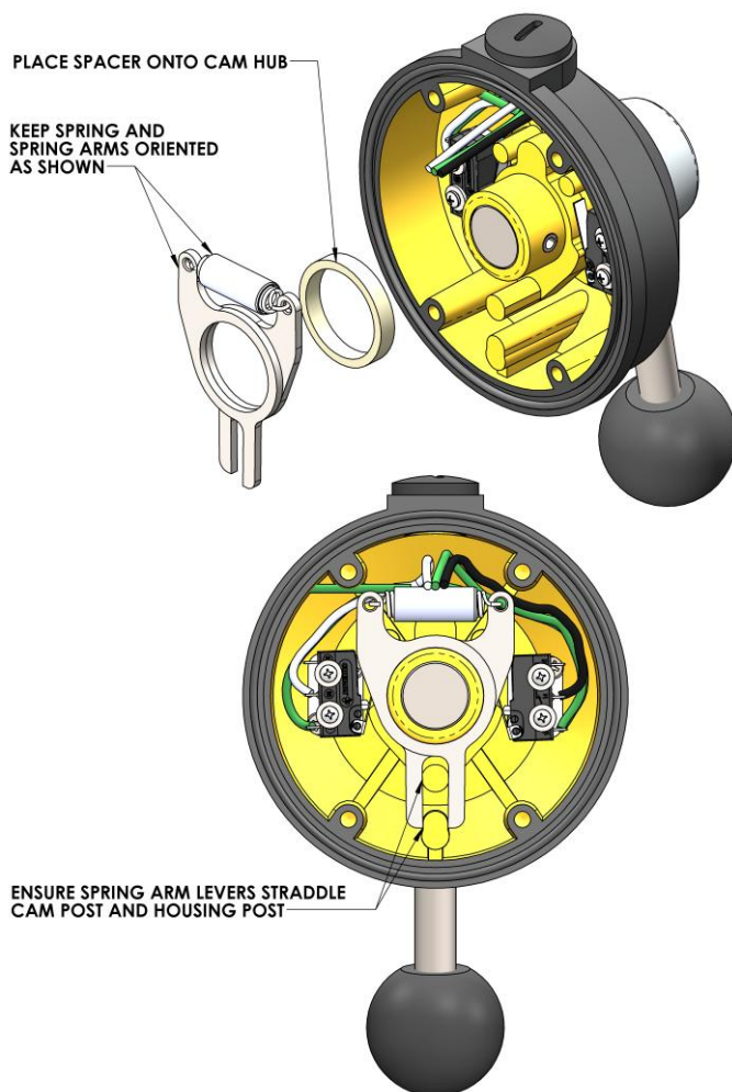
Figure 28: Installing spring assembly into jog housing.
