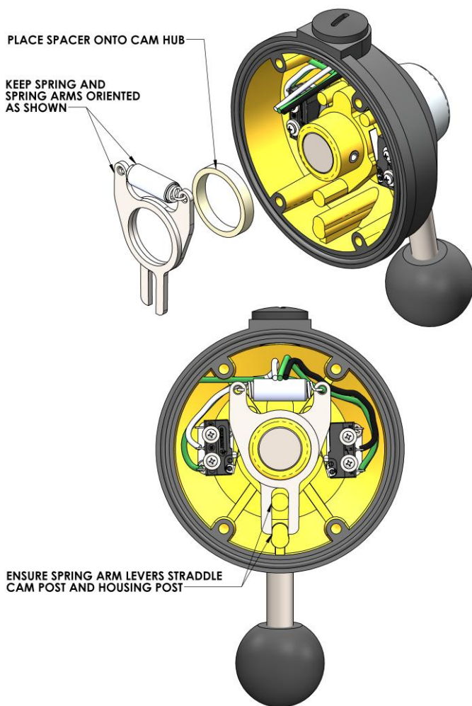
Figure 32: Installing spring assembly into jog housing.
