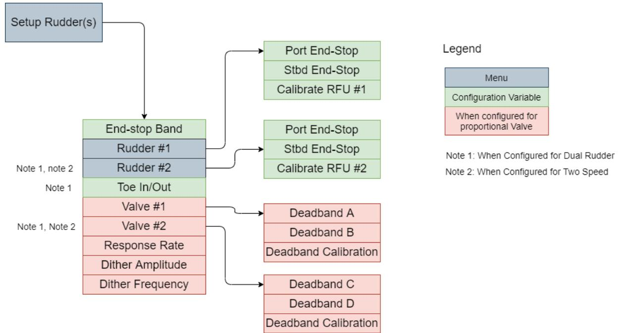
Figure 65: Setup Rudder(s)
