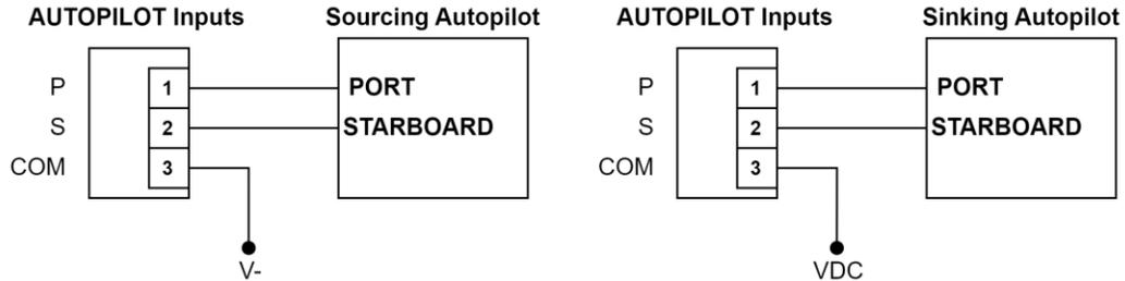
Figure 20: Autopilot Wiring for Autopilot with Solenoid Valve Outputs (Sinking or Sourcing outputs)
