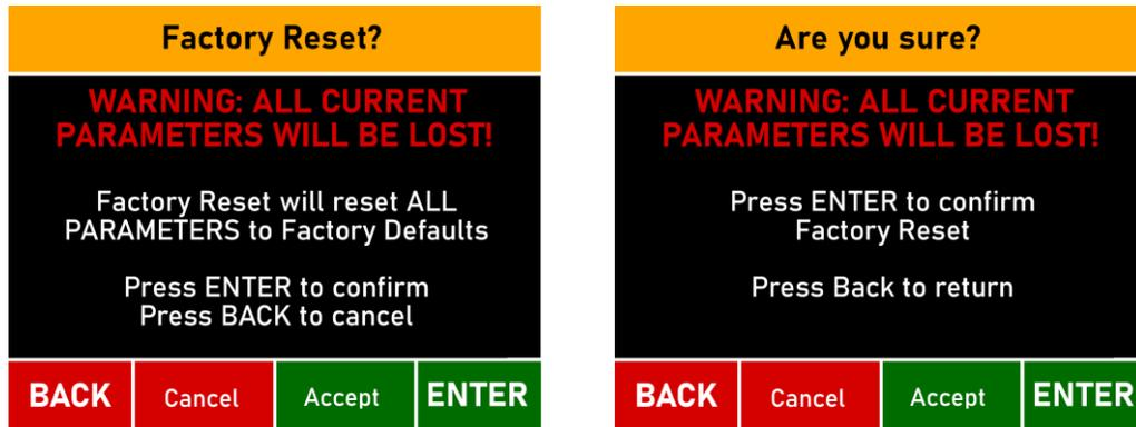
Figure 45: Factory Reset Confirmation Screen
