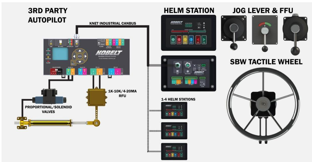
Figure 3: Steering System Block Diagram Render
