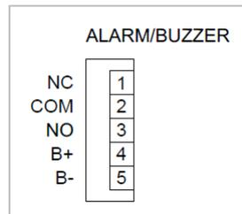
Figure 37: Electrical Connector for External Alarm Buzzer & Alarm Dry Contact
