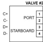
Figure 9: Electrical Connector for Valve #2 (Channels C/D)
