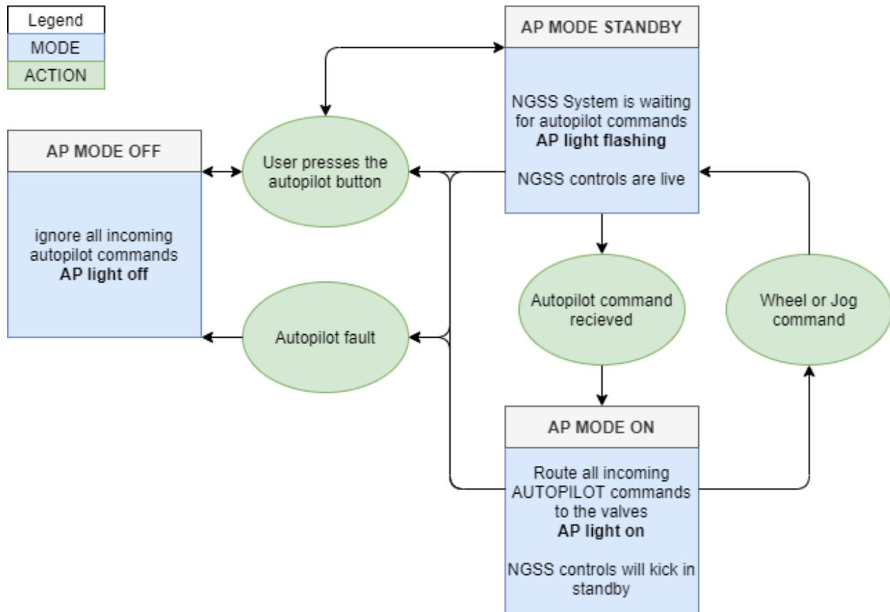
Figure 79: Autopilot Always Live State Diagram
