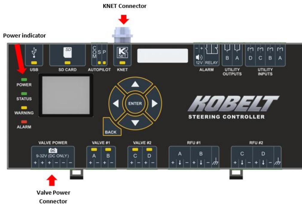
3. Remove all the connectors on the device.
