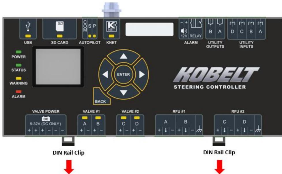
5. Remove the din rail clips from the housing
