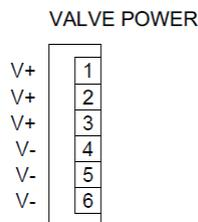
Figure 7: Electrical Connector for Valve Power
