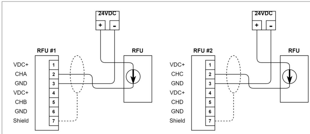
Figure 18: RFU Wiring for 2 Rudders with 2 Current Sensors
