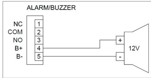
Figure 38: Wiring of External Buzzer Configuration
