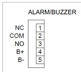
Figure 23: Electrical Connector for External Alarm Buzzer & Alarm Dry Contact
