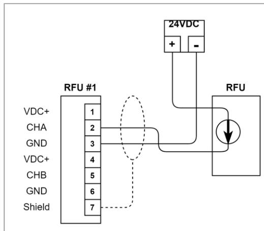
Figure 17: RFU Wiring for 1 Rudder with 1 Current Sensor
