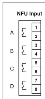
Figure 32: Electrical Connector for NFU Interface
