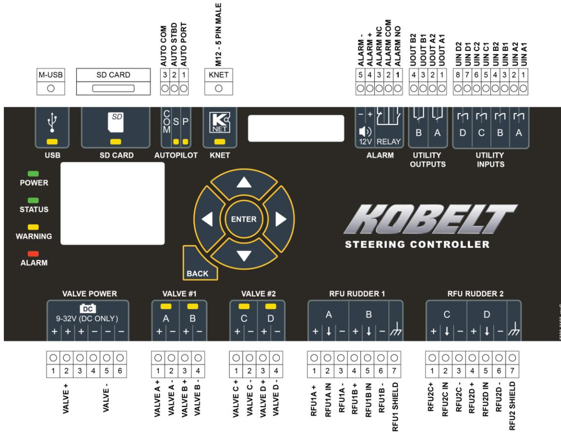
Figure 6: The Controller Wiring
