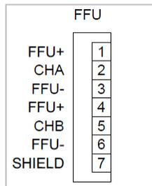
Figure 30: Electrical Connector for FFU Input Device
