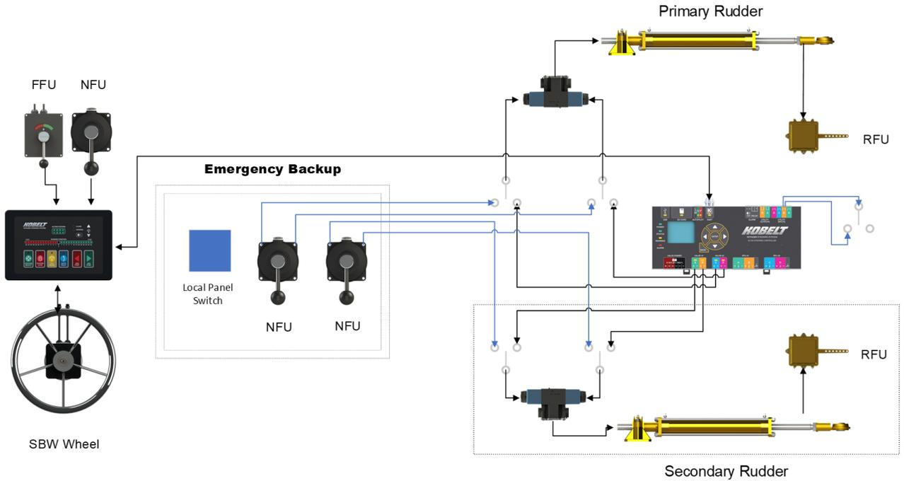
Figure 76: System with Local Emergency Backup Control
