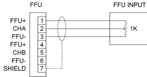
Figure 31: FFU Wiring with 1 Potentiometer Sensor
