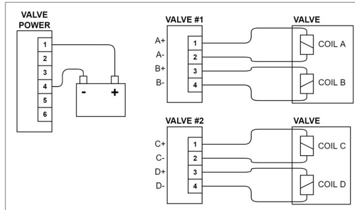
Figure 10: Valve Wiring for Solenoid Valves (4-Wire)
