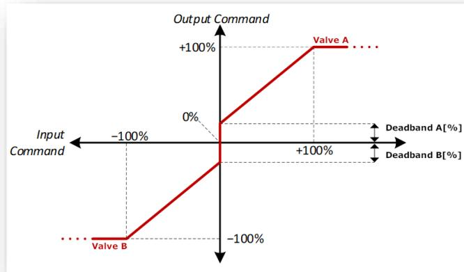
Figure 70:Valve Dead-band Graph
