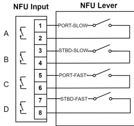
Figure 34: NFU Wiring for Two-Speed Jog Lever (8-Wire)
