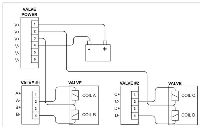
Figure 12: Valve Wiring for Solenoid Valves (Common Positive)
