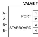
Figure 8: Electrical Connector for Valve #1 (Channels A/B)
