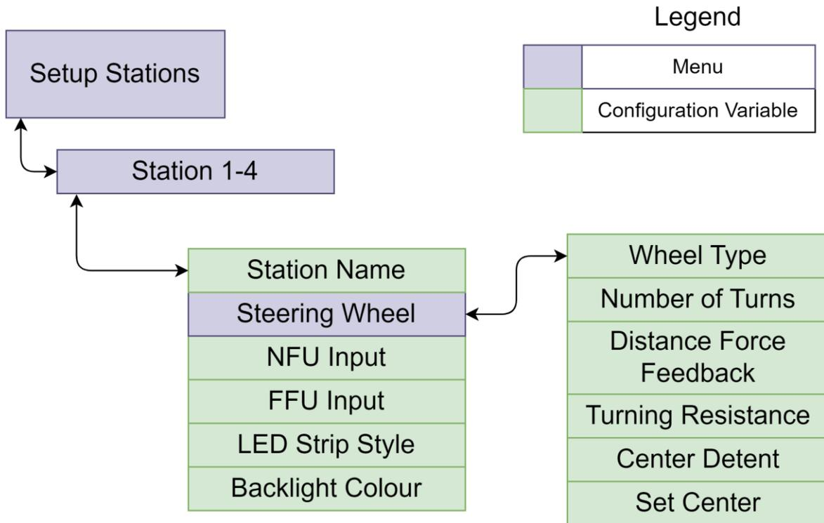
Figure 56: Steering Station Configuration Menu Overview
