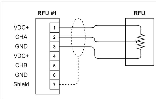
Figure 15: RFU Wiring for 1 Rudder with 1 Potentiometer Sensor
