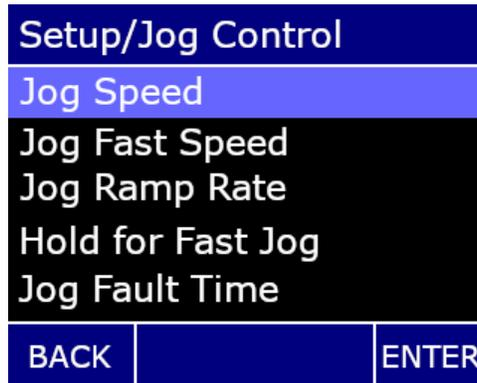
Figure 52: Setup Jog Control Screen
