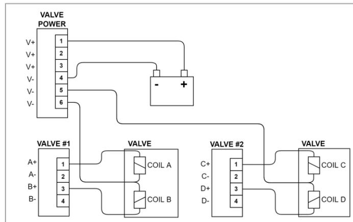
Figure 11: Valve Wiring for Solenoid Valves (Common Negative)
