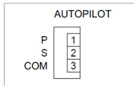
Figure 19: Electrical Connector for Autopilot Interface
