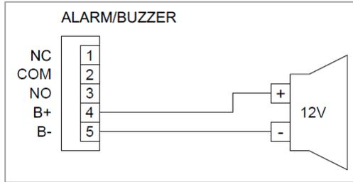
Figure 24: Wiring of External Buzzer
