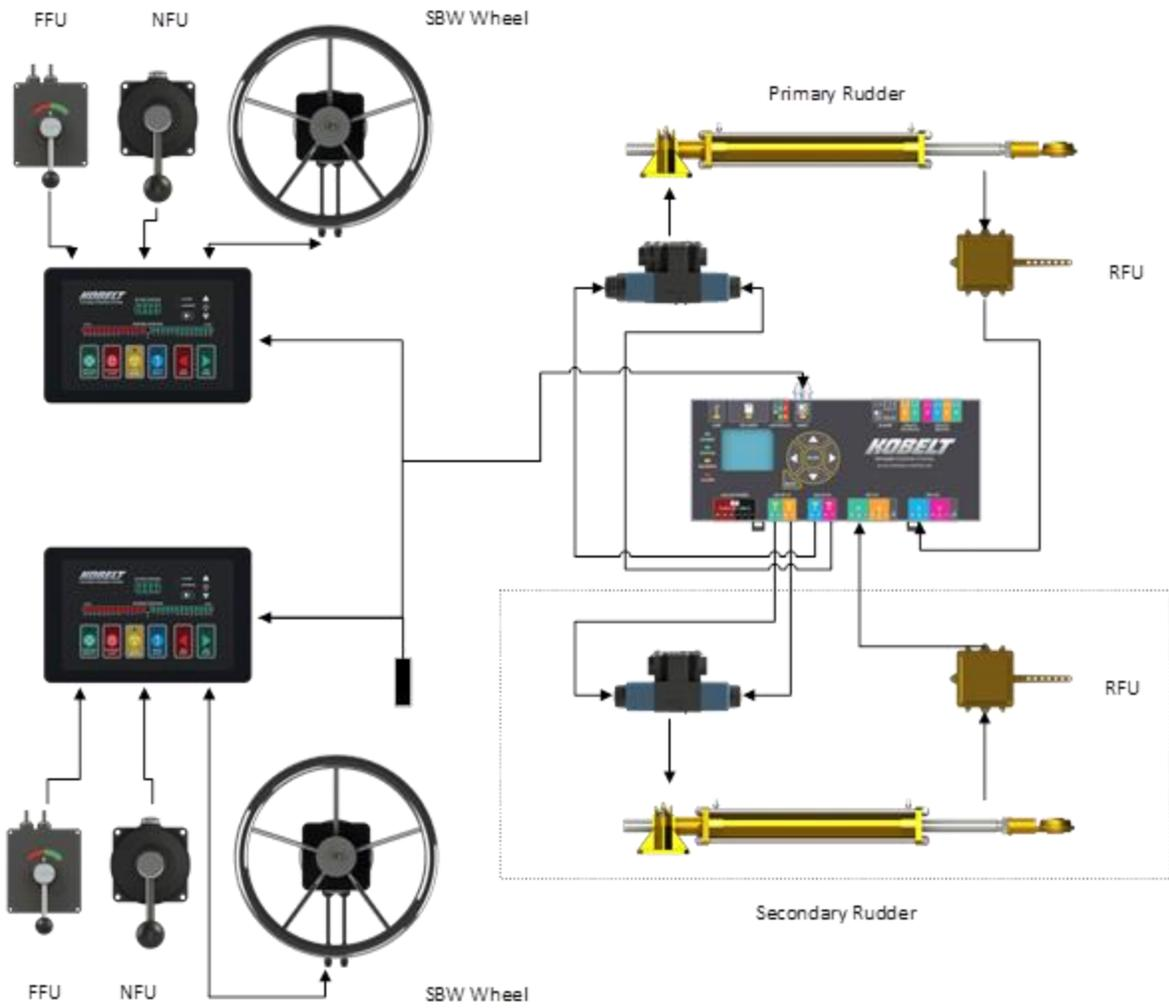
Figure 2: Dual Rudder Steering System Block Diagram (Simplified)
