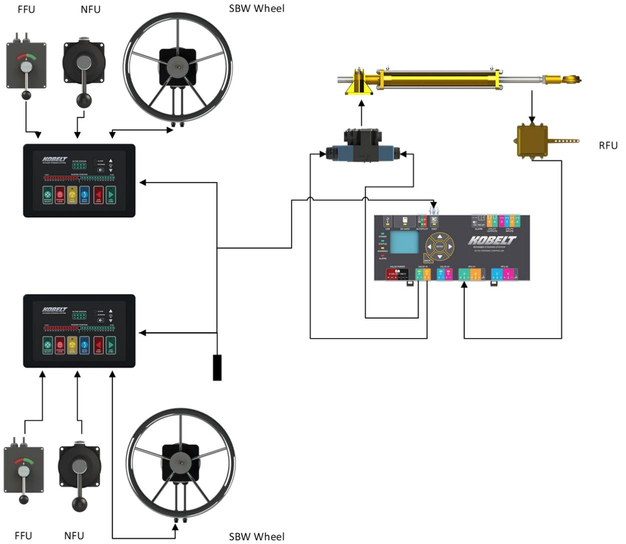
Figure 1: Single Rudder Steering System Block Diagram (Simplified)
