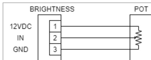
Figure 36: Brightness Wiring for Dimming potentiometer
