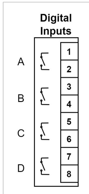
Figure 25: Utility digital inputs
