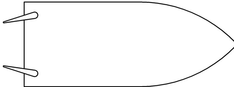
*Figure 67: Toe in configuration*
