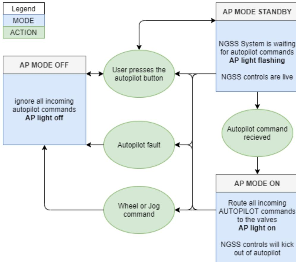
Figure 77: Autopilot Automatic Disengage State Diagram
