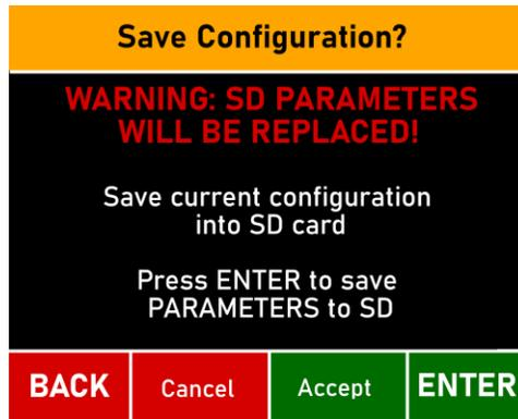
Figure 47: Save Configuration Confirmation Screen
