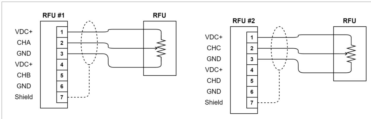
Figure 16: RFU Wiring for 2 Rudders with 2 Potentiometer Sensors
