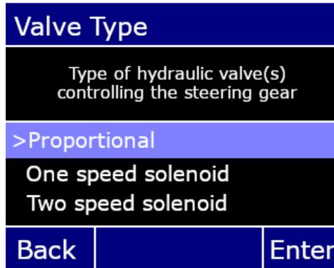
Figure 50: Set Valve Type Screen
