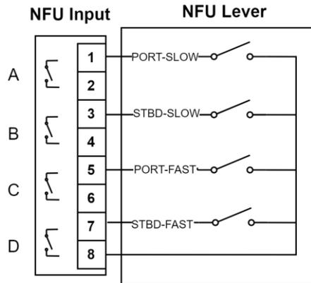
Figure 35: NFU Wiring for Two-Speed Jog Lever (Common Negative)
