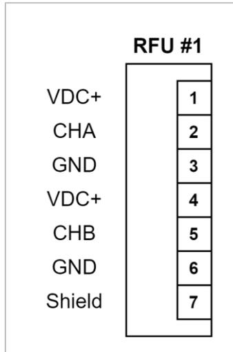
Figure 13: Electrical Connector for RFU #1
