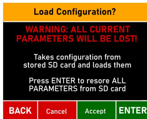
Figure 46: Restore Configuration Confirmation Screen
