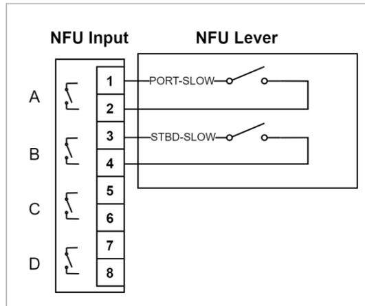
Figure 33: NFU Wiring for 1-Speed Jog Lever (Common Negative)
