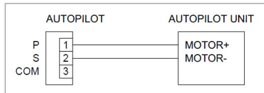
Figure 21: Autopilot Wiring for Autopilot with Reversing Pump Outputs
