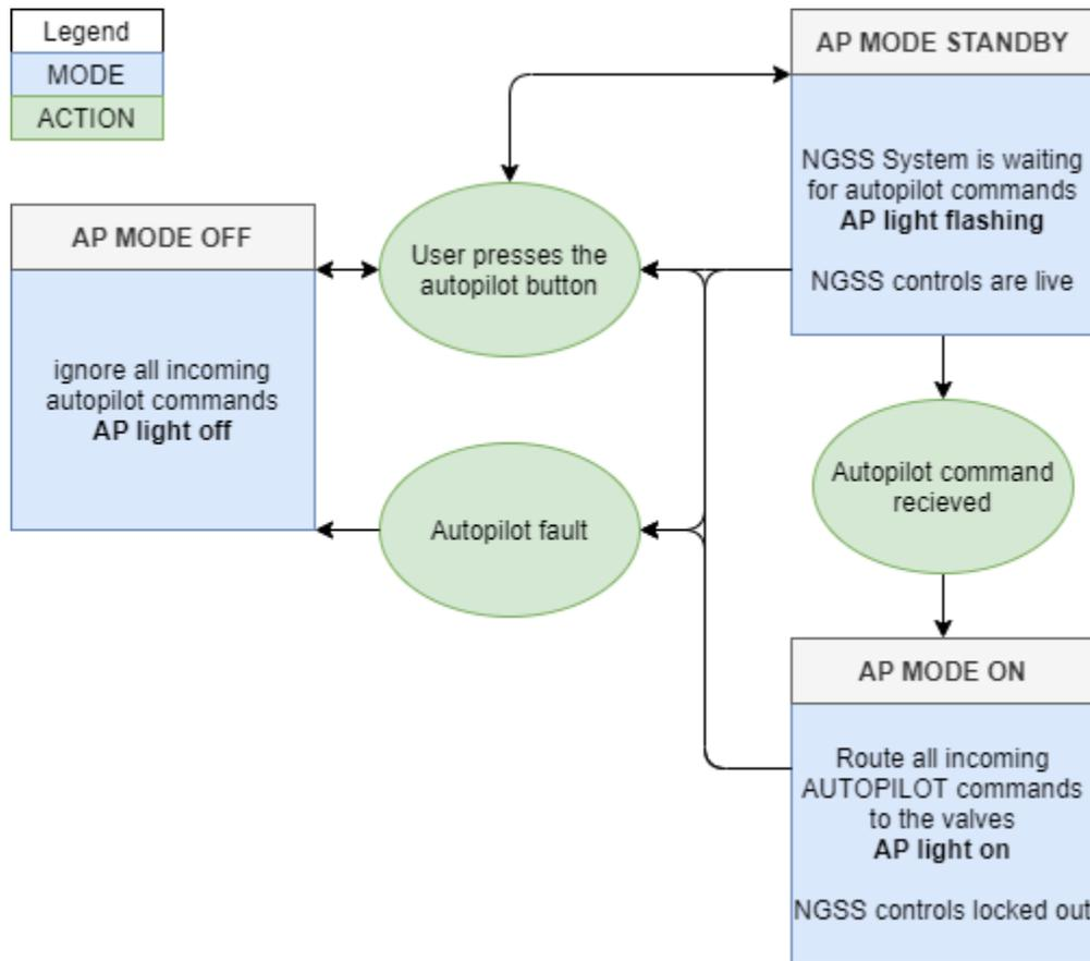
Figure 78: Autopilot Manual Disengage State Diagram
