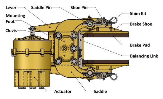
Figure 1: Caliper Brake Nomenclature
