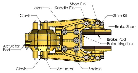
Figure 1: Caliper Brake Nomenclature
