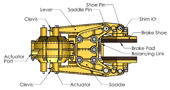
Figure 1: Caliper Brake Nomenclature
