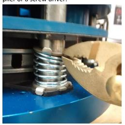
While holding the return spring compressed, slide the shoe radially outward. Repeat with the other retainer and lift the pad away.
