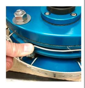
Starting with the mounting flange side pads first, push the pad retainer out of engagement with the backing plate. It may be necessary to use a brake spring plier or a screw driver.
