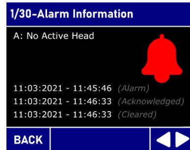
Figure 78: Fault Detail Screen
